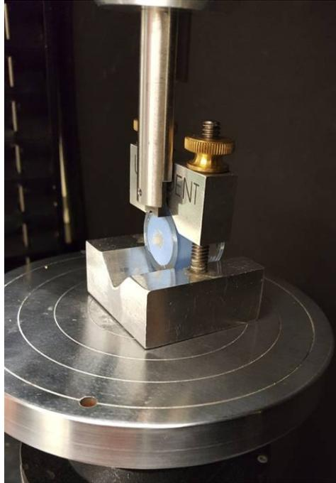
FIGURE 9. Shear bond strength testing.
