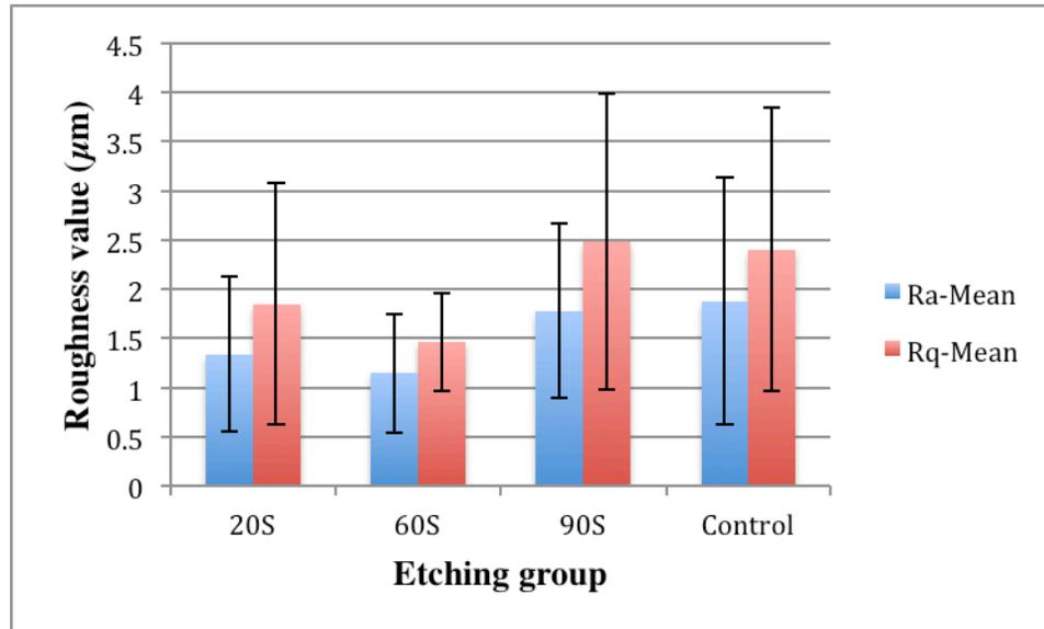
FIGURE 11. Surface roughness means and respective  $\pm$  SD of experimental groups.
