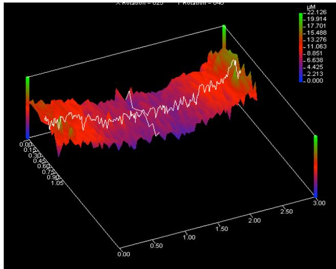
FIGURE 15. Representative non-contact profilometry scan of 60-s etched ceramic group.
