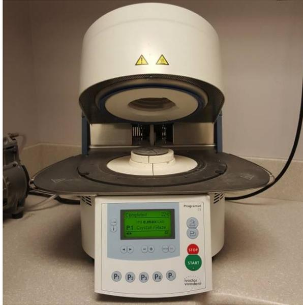
FIGURE 2. Vacuum pump furnace (Programat CS/CS2).
