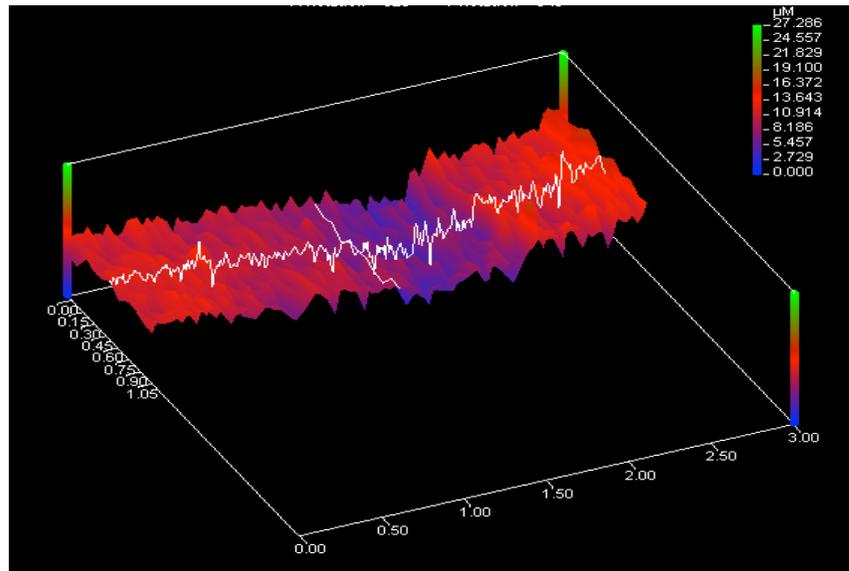
FIGURE 14. Representative non-contact profilometry scan of 20-s etched ceramic group.
