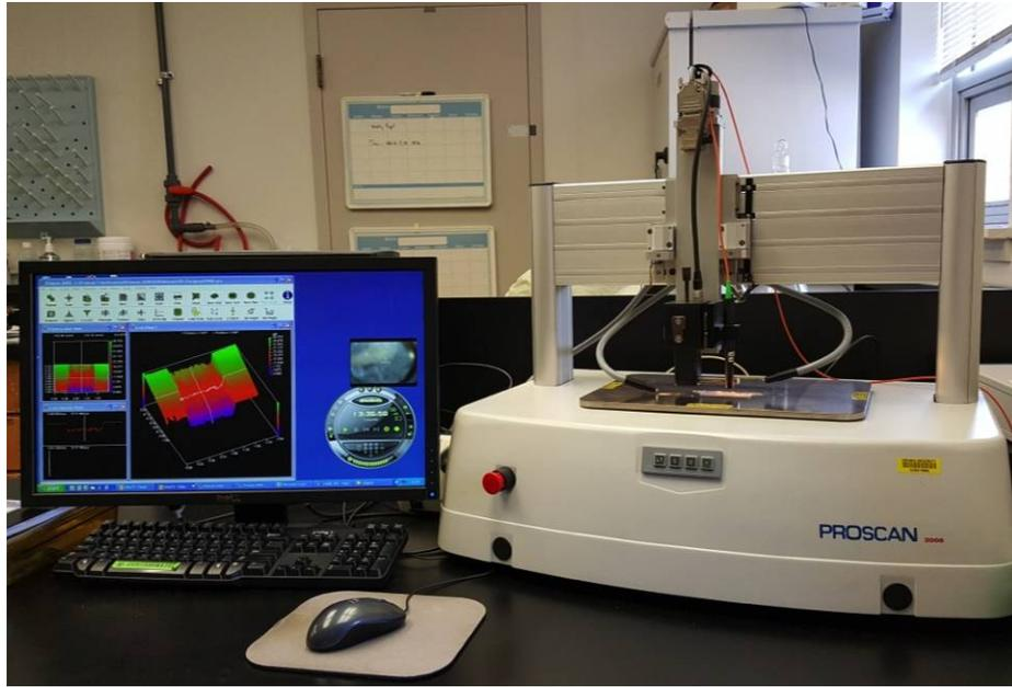
FIGURE 6. Non-contact optical profilometer (Proscan 2000).
