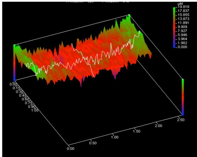
FIGURE 16. Representative non-contact profilometry scan of 90-s etched ceramic group.
