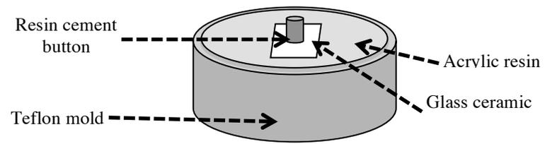
FIGURE 7. Schematic representation of mounting specimens for SBS testing.
