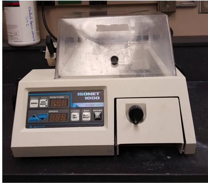
FIGURE 1. Isomet 1000, a cutting machine.
