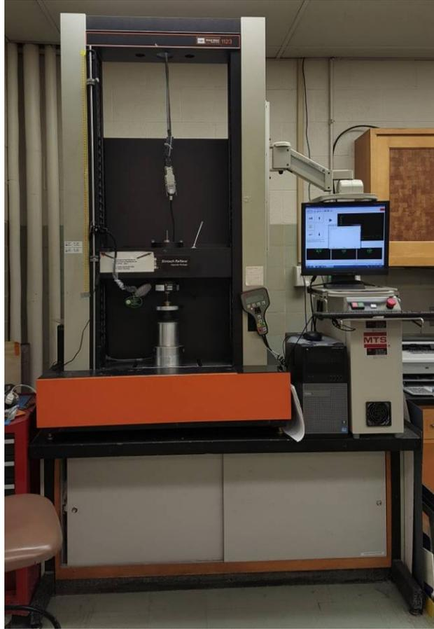
FIGURE 8. Universal testing machine (MTS).
