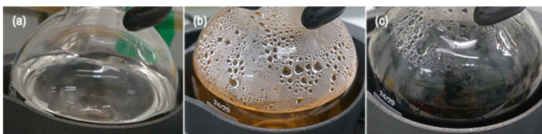
Figure 2 Photographs of glycerol heated under the same condition as the exfoliation process, (a) before and (b and c) after heating for (b) 90 min, (c) 3 days.
