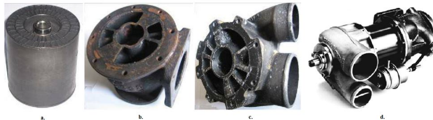
Figure 1.2. Components of Complex Pressure Wave Supercharger. a. rotor; b. hot stator plate; c. cold stator plate; d. Complex unit [27]
