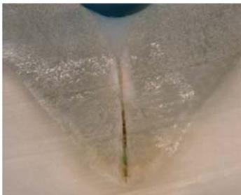
FIGURE 13R. Sealant penetration.
