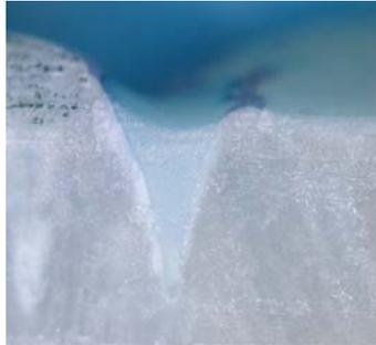
FIGURE 13B. Sealant penetration.
