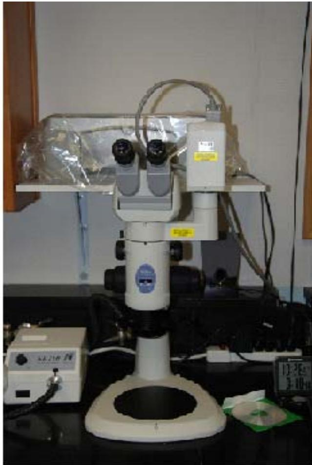
FIGURE 11. Image of Nikon SMZ 1500 Microscope used to take images.
