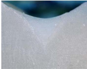
FIGURE 13J. Sealant penetration.
