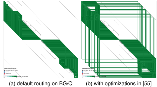
Figure 12: Matrix MPI I/O communications with 512 compute nodes using 16 ranks/node. (a) Network traffic is localized in two regions. Approach in (b) tries to use many under-utilized links.
