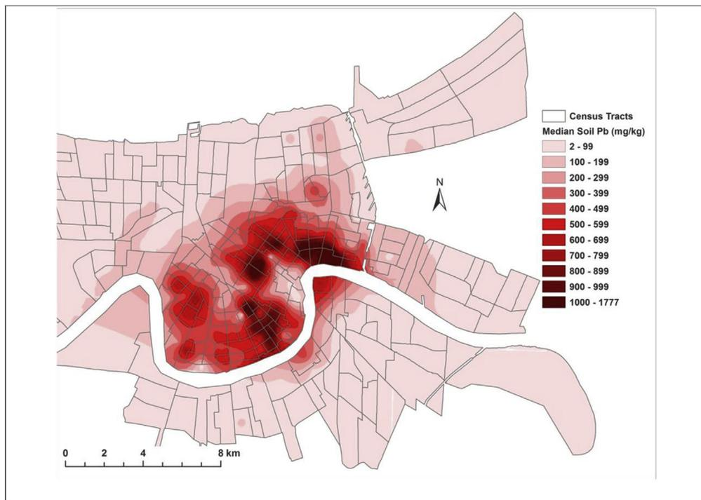
**Fig. 1.** Typical urban inner city soil lead distribution as shown in pre-Hurricane Katrina New Orleans, Louisiana, USA. The low lead soil area surrounded by soil with extreme lead values is the Central Business District where surface soil is covered by pavement and not readily available (Gonzales CR, Powell ET, Mielke HW, unpublished original for this review).
