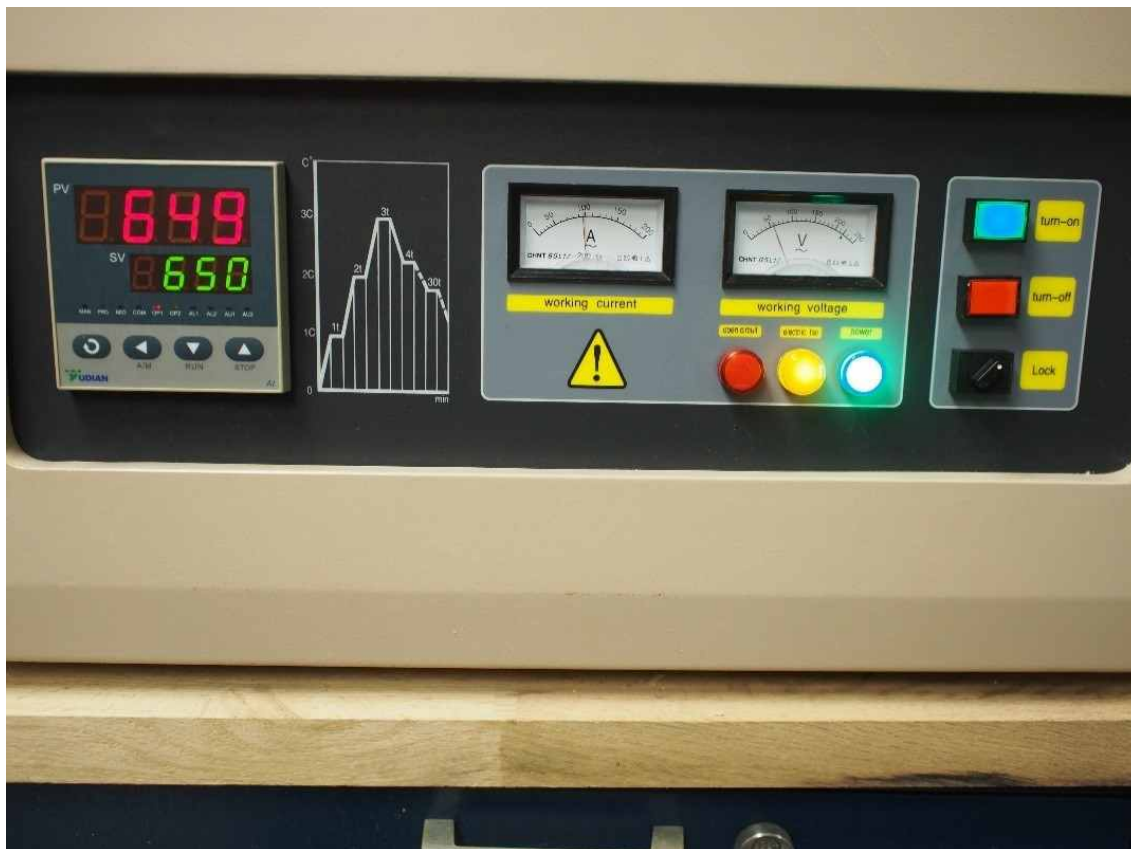
Fig. 2.15. Control panel of tube furnace.
