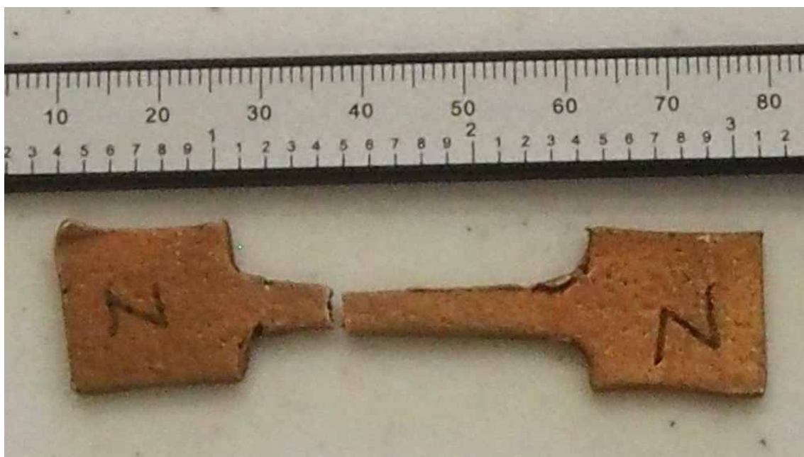
Fig. 3.5. Molded specimen after break.
