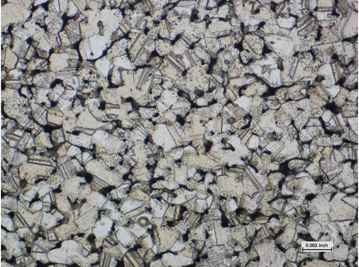
Fig. 5.1. 200x magnification of Molded BMC.
