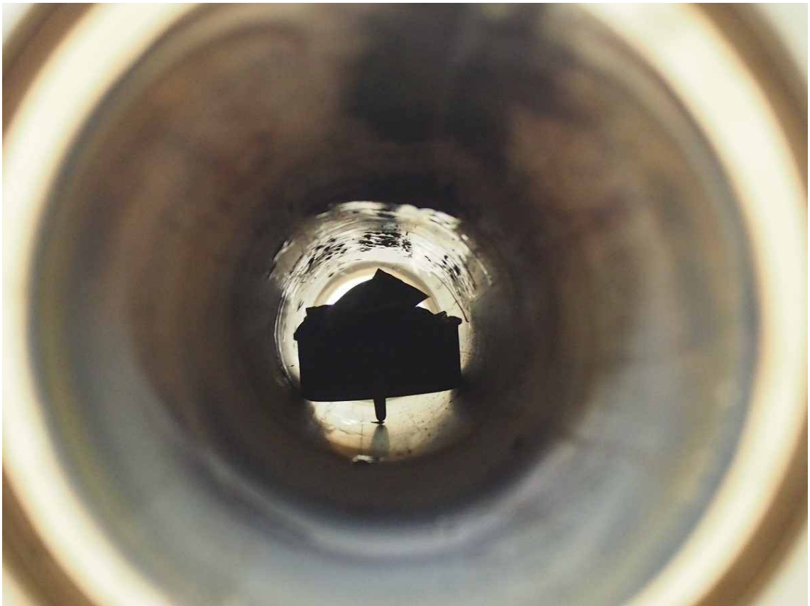
Fig. 2.14. Stainless steel tray sits in the center of the tube furnace.
