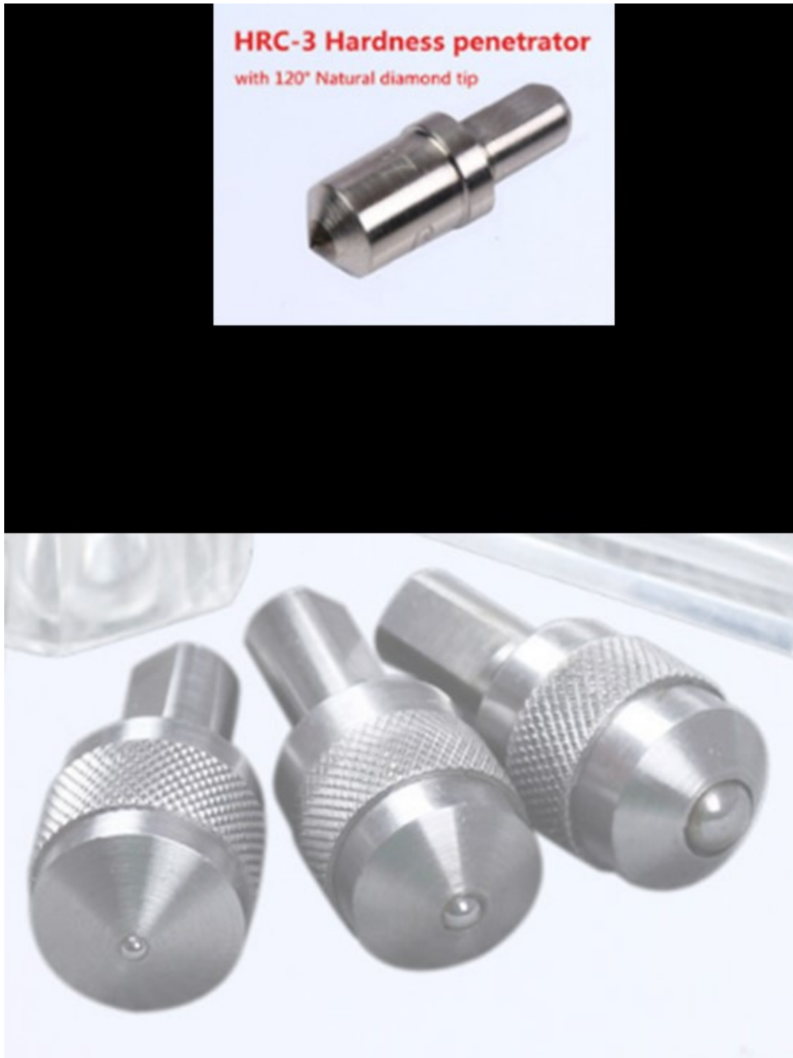
Fig. 4.2. A diamond tip and other tips that use different size balls for hardness testing.
