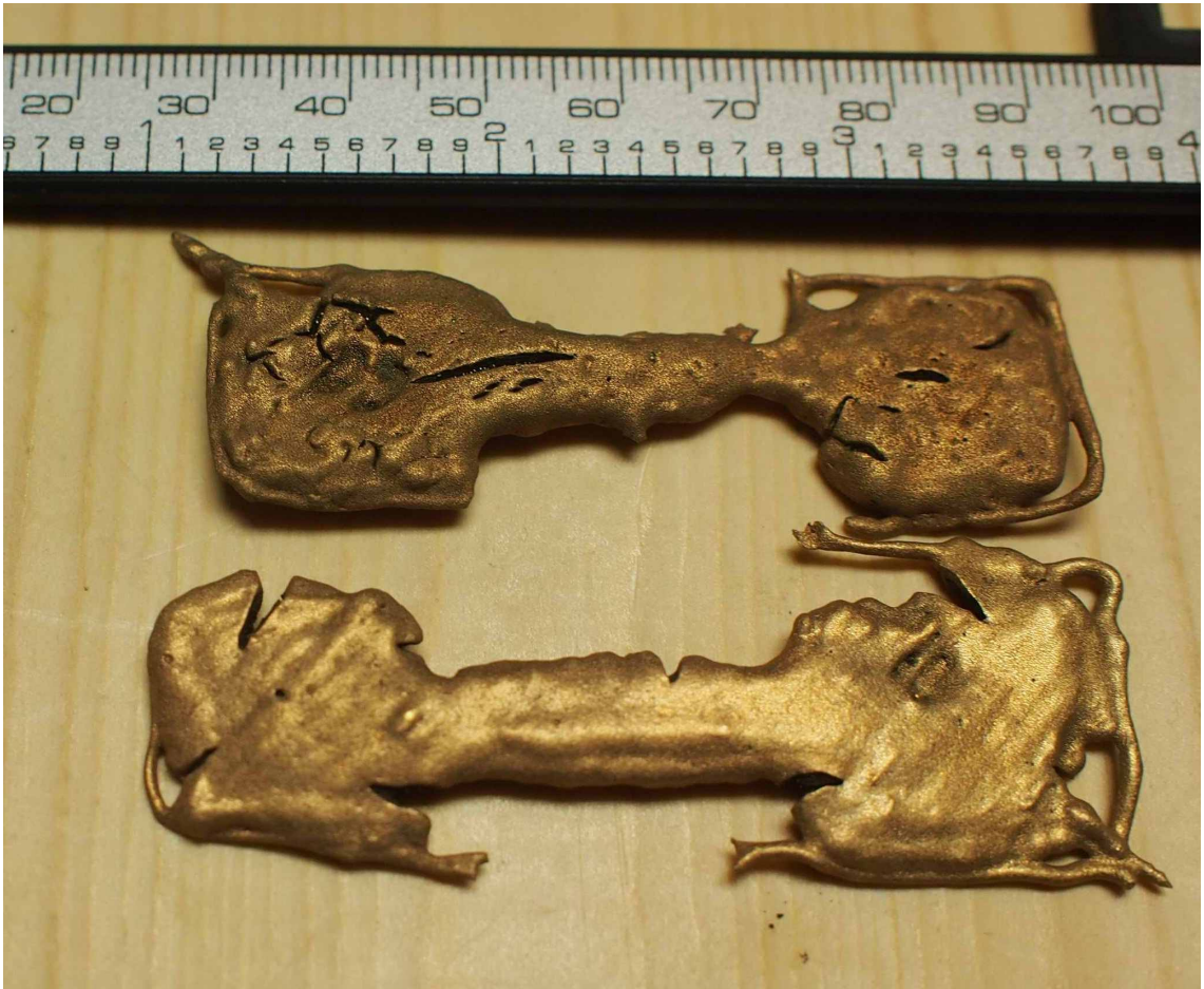
Fig. 2.12. 3D printed specimens after firing.
