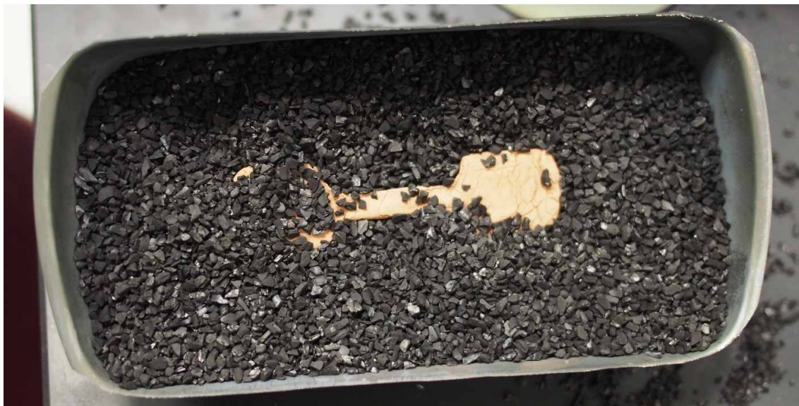
Fig. 2.16. Stainless steel dish with charcoal and bronze tensile bar.
