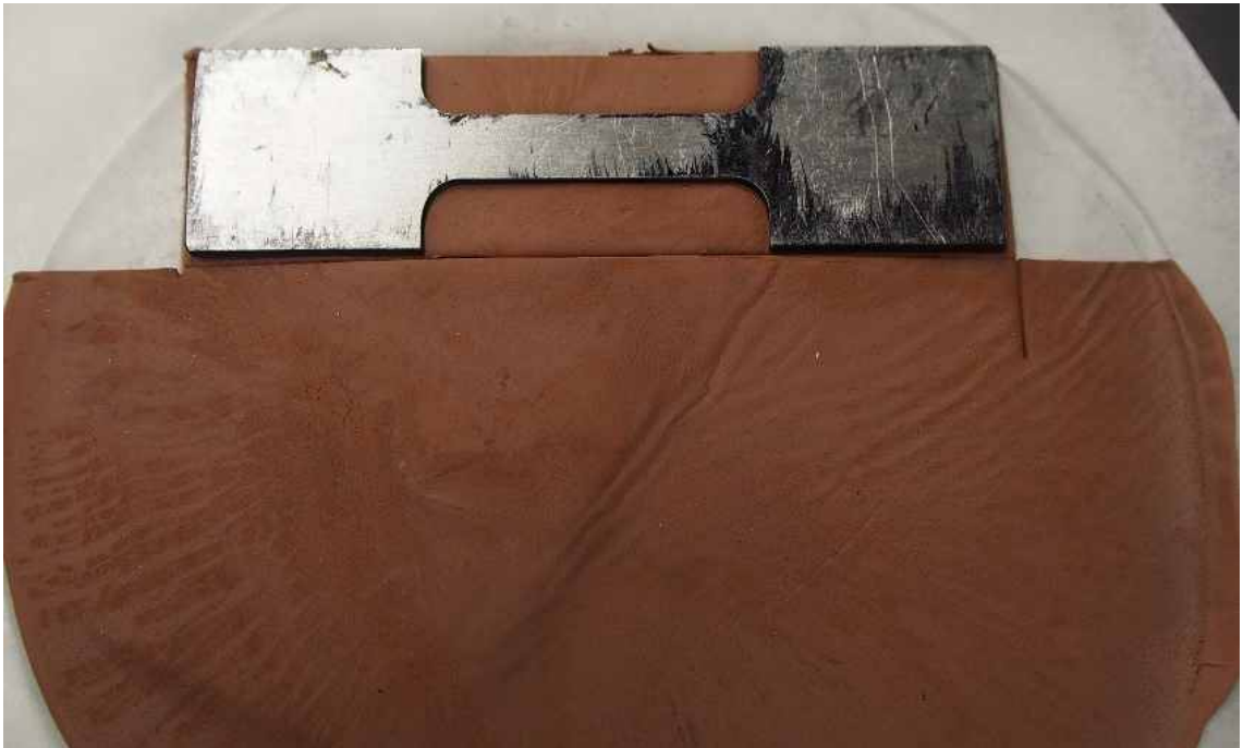
Fig. 2.10. Tensile strip partially cut out from the clay.
