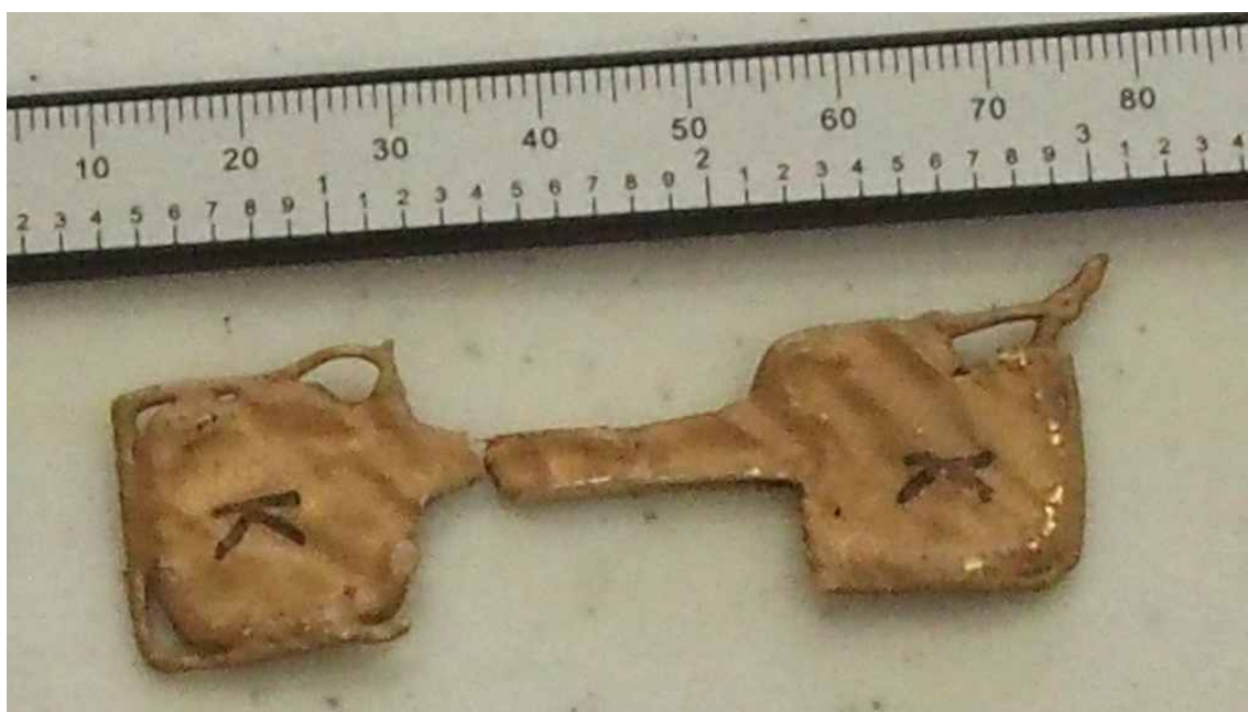
Fig. 3.6. Printed specimen after break.
