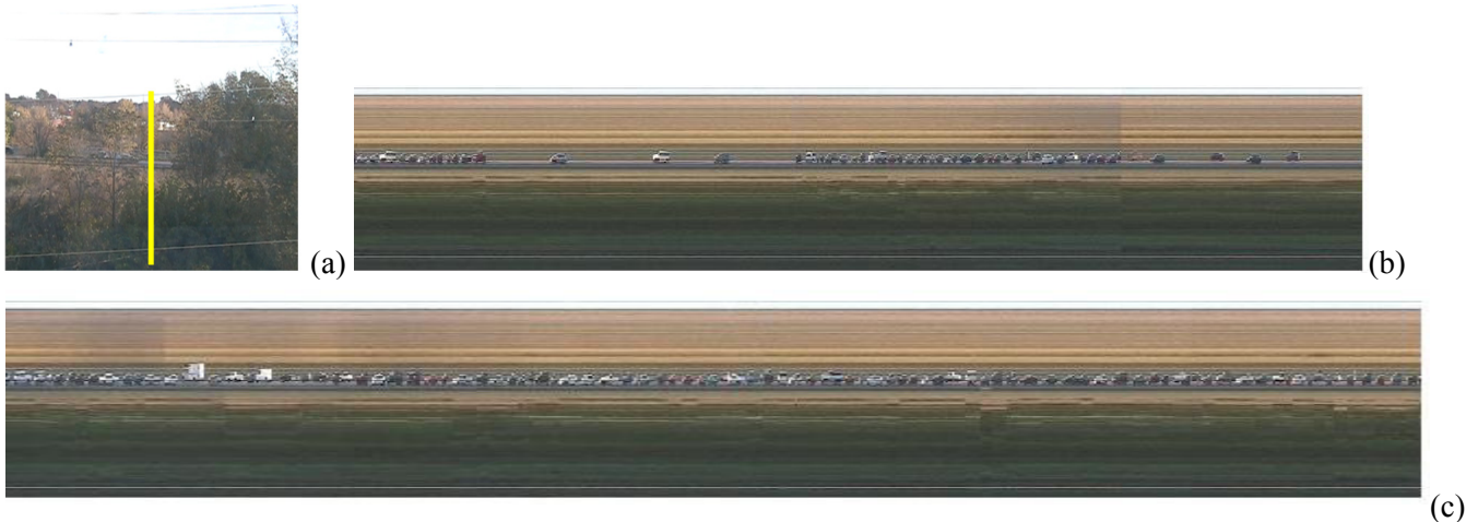
Figure 13: Detecting dynamic objects in real time. (a) Field of view with a sampling line intersecting a distant road. (b) A section of temporal profile with vehicles and their times of arrival. (c) Detected vehicles and their summarized sections transmitted to a data center.
