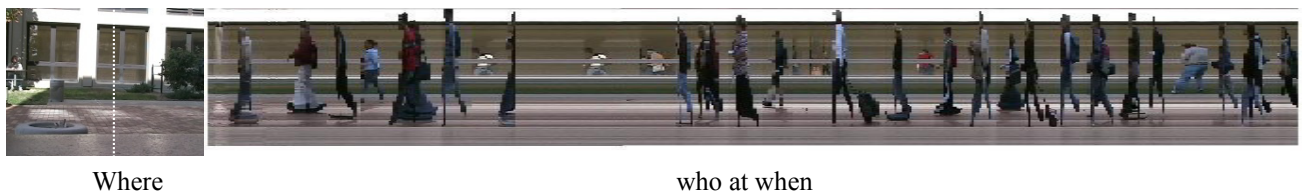
Figure 2: A sampling line in the frame and its generated temporal profile. (Left) A frame with the vertical sampling line depicted. (Right) Profile collected from the sampling line recording people both at front and in the hallway behind the window.
