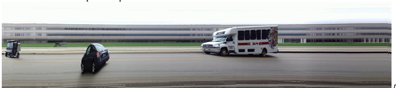
(b) The resulting temporal slice cut in the corrected video near the left margin. The shrinking at the middle range of the clip is due to the changes in the vertical flow component. The temporal slice displays the different vehicles passing the sampling line.
