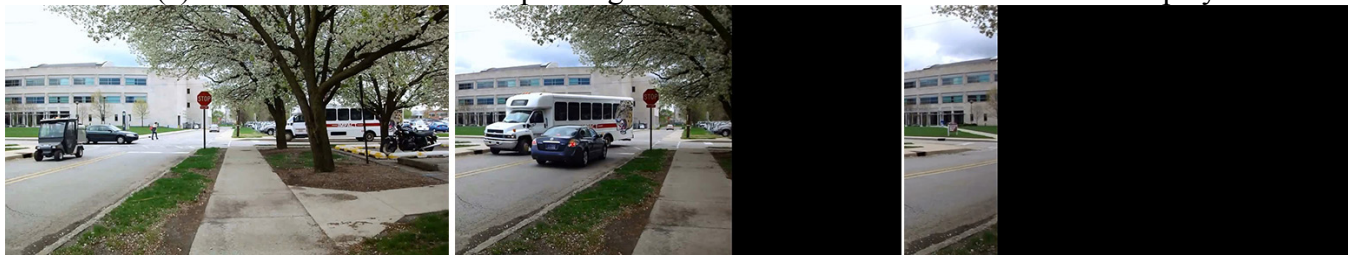
(b) Static video created by compensating the panning motion. Dynamic field of view is pasted into the initial video frame automatically.
