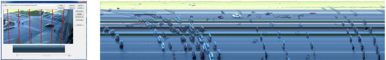
Figure 21: Global motion in temporal profile generated at an intersection. Series of copies of cars are extracted when they move from right to left in the view (from transparent to opaque in profile). The time delays are shorter for cars than for pedestrians because of a faster speed of cars in the view.
