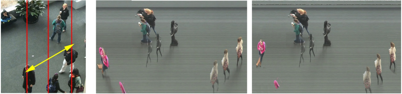
Figure 8: A simple local skew deformation to reduce the proportion of depth stretching edges for better shape understanding in the temporal slice. (Left) A frame with red sampling lines and yellow v direction, (Middle) three temporal slices combined, and (Right) locally rectified pedestrians based on detected areas of passing targets.
