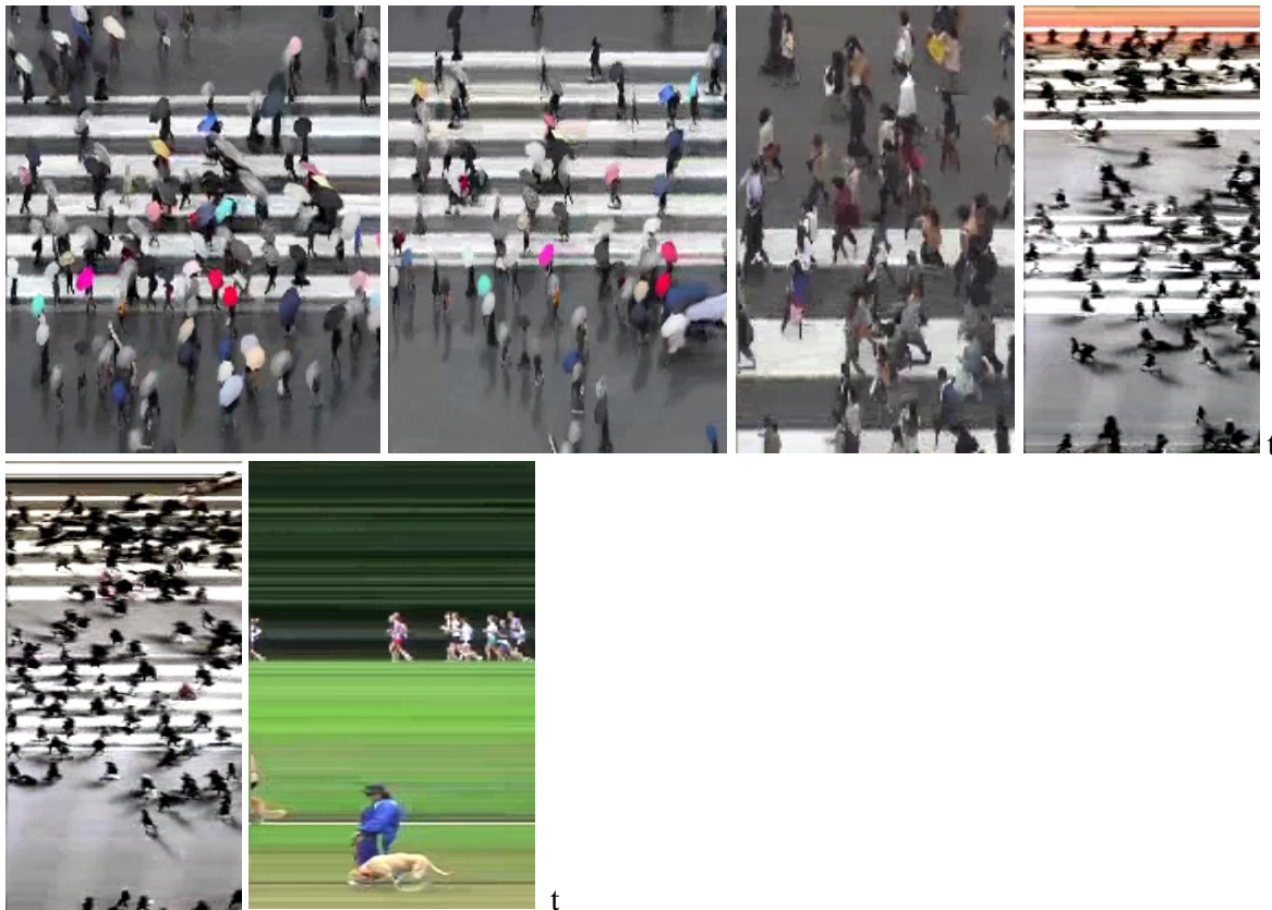
Fig. 4 (b) Vertical sampling line obtained temporal slices. The time axes are horizontal. Block effect is visible in some slices due to the lousy video compression based on temporal coherence.
