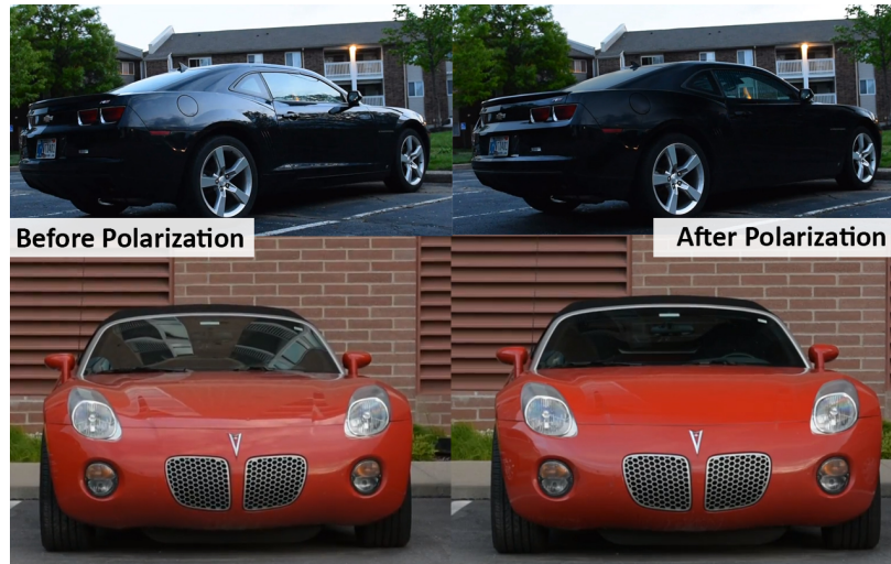
Figure 3.10. An illustration of how the circular polarizing filter/Linear (CPL) camera filter used to reduce reflections and glare [3]
