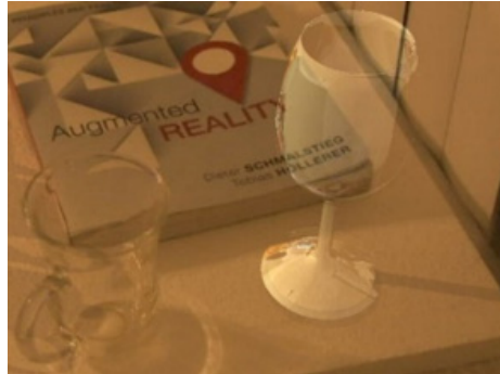
Figure 6.2. The effect of image-based Fresnel on the glass [2]
