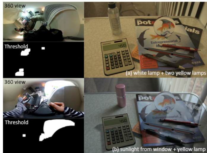
Figure 8.2. Initial results, each case has: live 360 view, threshold mask of direct illumination detection, final result [1]
