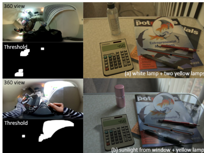
Figure 3. Experiment results, each case has (1) live 360° view, (2) threshold mask of direct illumination detection, (3) final result.
