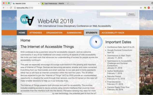
Figure 6. The Adaptive Bubble Cursor in action. The cursor's selection area grows in response to an increase in detected pointing errors. The larger size makes it easier to select objects close to the cursor. In the adaptive mode, the size and selection area of bubble cursor change in response to pointing error detection. The user can specify whether the selection area of the bubble cursor should be visible or hidden.
