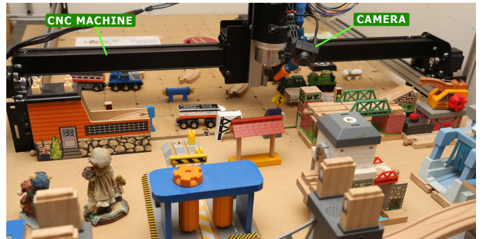
Fig. 14: Experimental setup showing a camera mounted on a CNC machine allowing us to capture ground truth information. Camera mounted on a CNC machine
