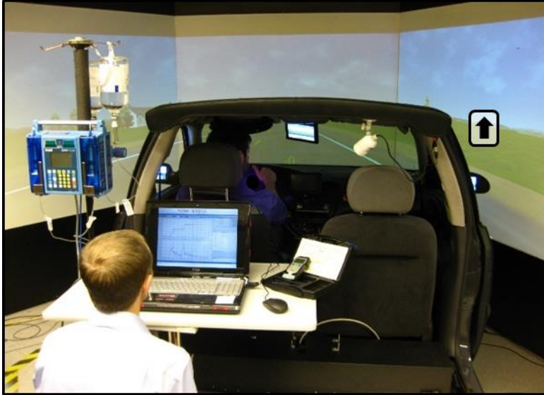
Figure 1: Apparatus employed in this study. The TASI DS-600c Driving Simulator is shown from the rear along with the CAIS apparatus (alcohol infusate, computer-controlled infusion pump, laptop with PBPK model embedded in CAIS software and breath alcohol concentration meter). The driver's thumb is pushing a button mounted on the steering wheel to indicate the perceived direction of the arrow on the pseudo-road sign moving past him with the environment.
