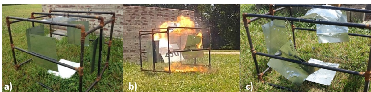
Figure 3: Photographs of the PVC pipe bomb trial set-up, a) prior to; b) during; and c) following initiation of the device.
