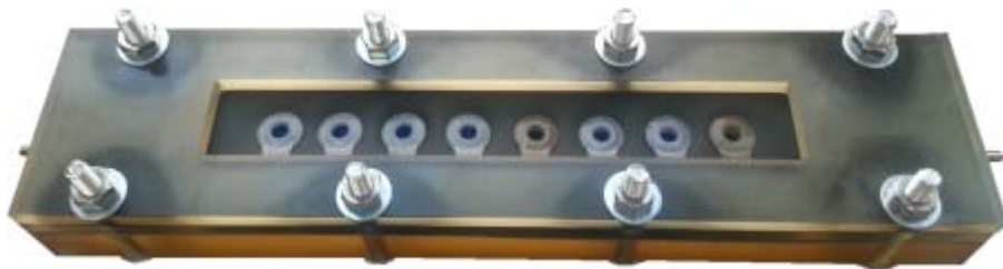
Figure 2. Proprietary Modified Robbins Device with TEPs.
