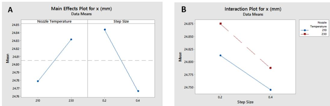
**Figure 3** A- Main effects plot for nozzle temperature and step size; B- Interaction plot for nozzle temperature and step size.
