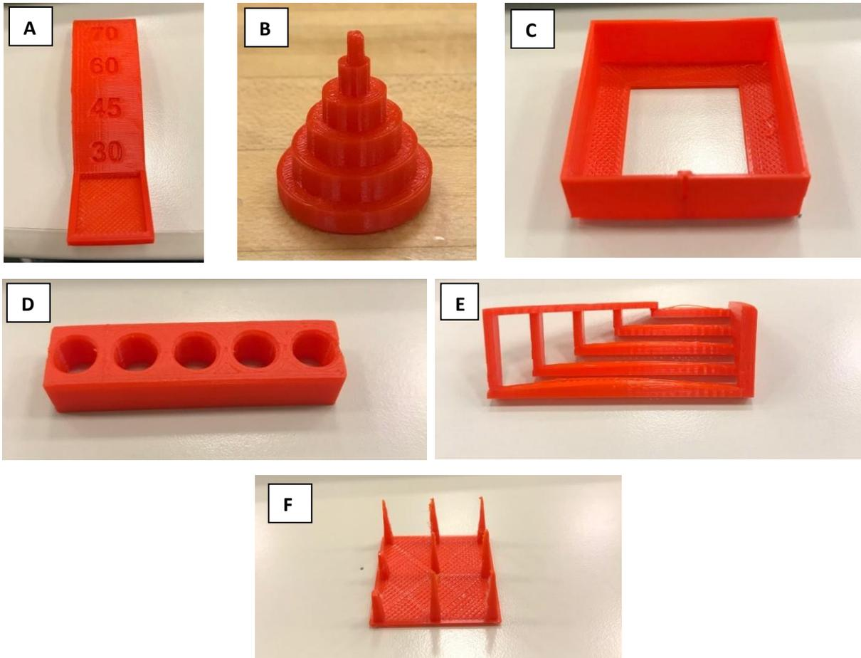
**Figure 1** Printed parts as per different calibration aspects. (A) Overhang performance; (B) Dimensional accuracy; (C) Mechanical resonance in XY; (D) Negative space tolerance; (E) Bridging performance; (F) Fine positive space feature performance.
