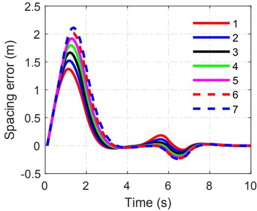
Fig. 5. Spacing errors for the platoon under PF topology in Scenario 1.
