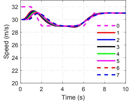
Fig. 6. Control effects of velocity for the platoon under PF topology in Scenario 2.
