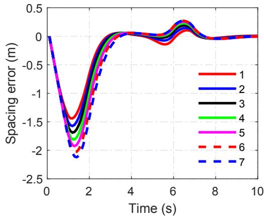
Fig. 8. Spacing errors for the platoon under PF topology in Scenario 2.
