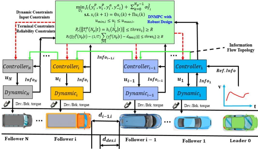
Fig. 1. Overall structure of DN MPC for heterogeneous platoon considering robust design and reliability-based design under PF topology.
