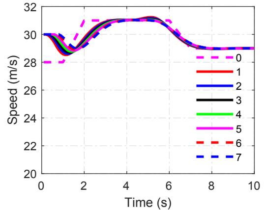
Fig. 3. Control effects of velocity for the platoon under PF topology in Scenario 1.
